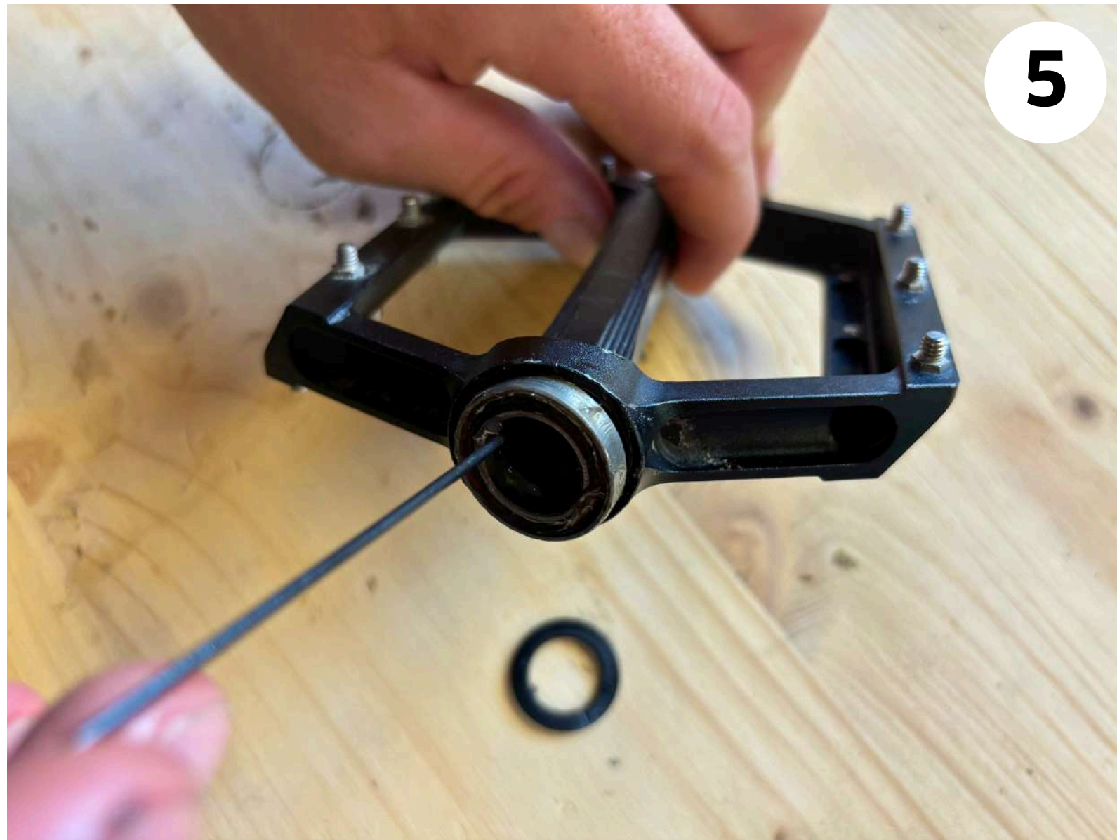
Take the spring washer and the bearing out of the pedal body on the other side.
