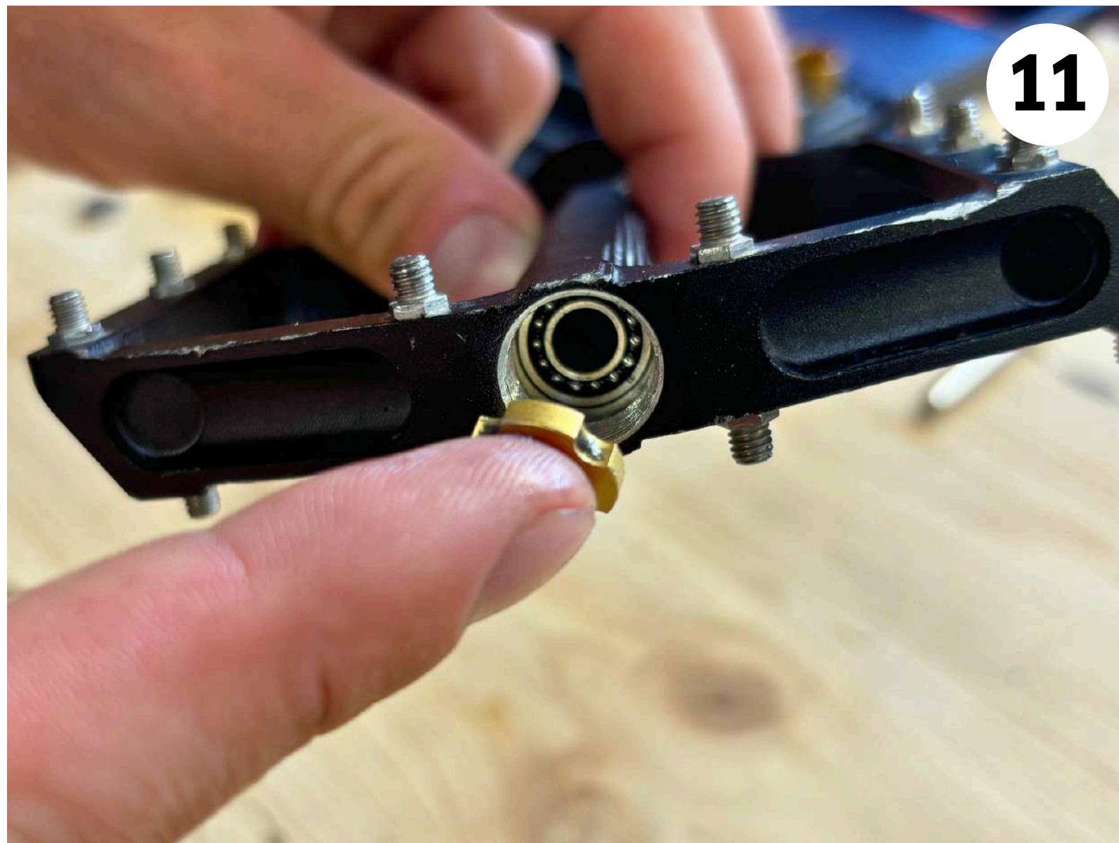
Insert the brass washer on the outside of the pedal body.
